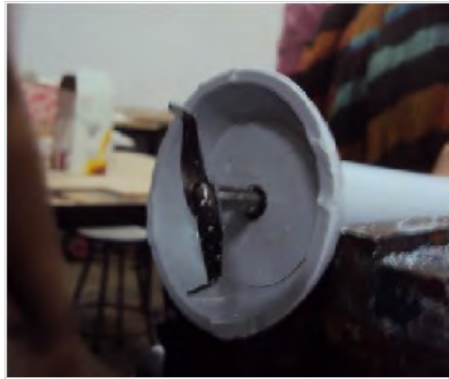
saw off border of the blade
