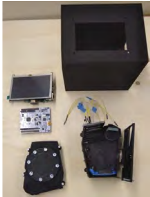
Figure 4: Completed Merlin spectrometer with outer case, nucleo, Raspberry Pi and LCD display.
