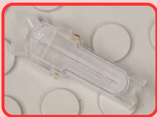
Figure 4. Dialysis membrane used in our experiment procedure. 10000 kDa molecular cut-off
