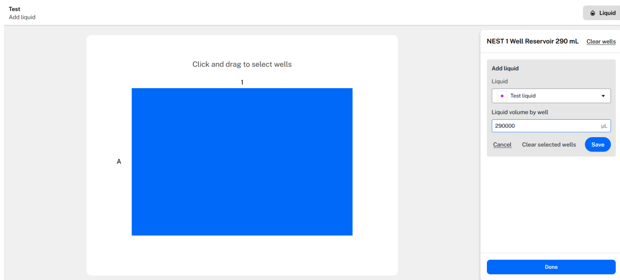
Figure 3. Opentrons interactive user interface for online design of protocols, specifically definition of liquid cultures.
