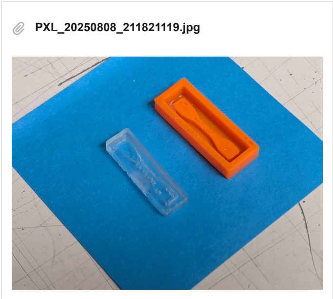
PDMS mold taken out from oven. Note there are minor bumps on the mold due to imperfections in the 3d print.
