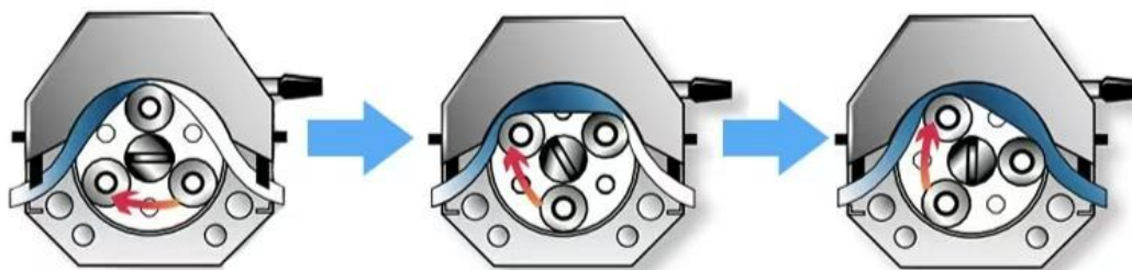
Figure 13 Working Principle of the Peristaltic Pump
